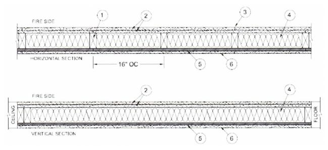
1. **Framing Members\*** — Pressure-treated, fire-retardant Wood Studs - nom. 2 by 4 in., spaced 16 in. OC in. effectively fire stopped. As an option, nominal 2 by 6 in., spaced 24 in. OC effectively fire-stopped.
